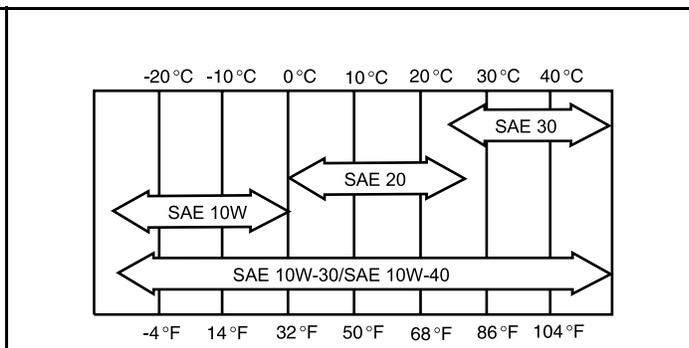
214 **Figure 29 Oil Viscosity Chart – Diesel Vehicles**
