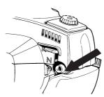
Choke: Set the choke control in the choke position.
