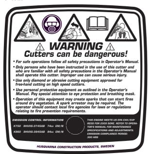
The Emissions Compliance Period referred to on the Emission Compliance label indicates the number of operating hours for which the engine has been shown to meet Federal emissions requirements.
