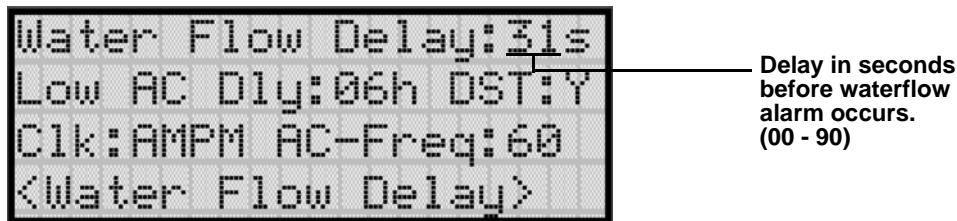
Figure 7-16 Water Flow Delay Programming Screen
