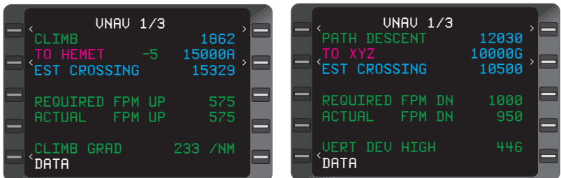
Progression of Vertical Waypoints from Climb to Path Decent on VNAV 1/1 Figure 2-41
