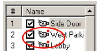
Fig. 5-4. A Red Dot Is Added to the Icon of a Camera that Is Recording.
