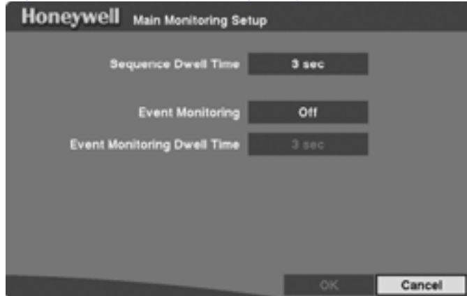
Figure 3-49 Main Monitoring Setup Screen
