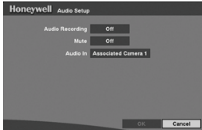
Figure 3-30 Audio Setup Screen
