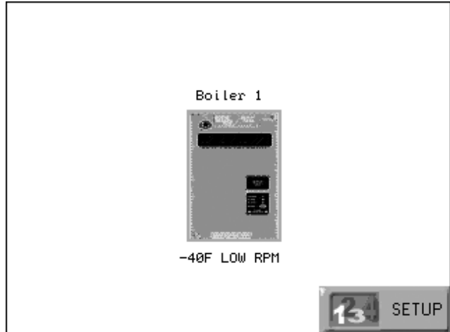
Fig. 6. S7999B Home page (Boiler 1 in normal operation).
