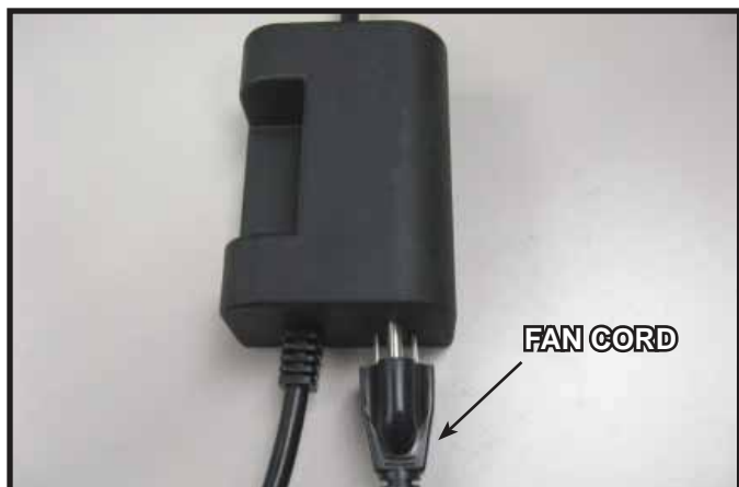
Figure 5. Plug Fan into AUX200 Module
