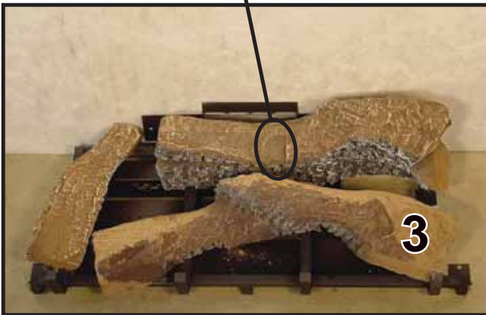
LOG #3 (SRV768-704): Position log #3 onto grate such that the tab D fits into the slots on bottom surface of log and the right back side of log is flush against tab E.
