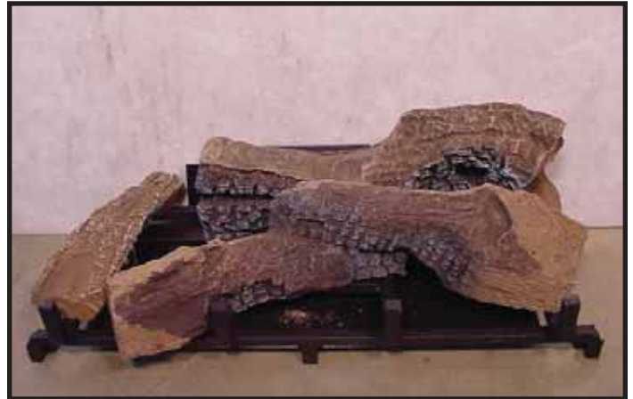
LOG #3 (SRV768-704): Position log #3 onto grate such that the tab D fits into the slots on bottom surface of log and the right back side of log is flush against tab E.
