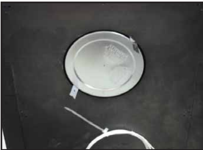
Figure 9.6 Remove the seal cap.
