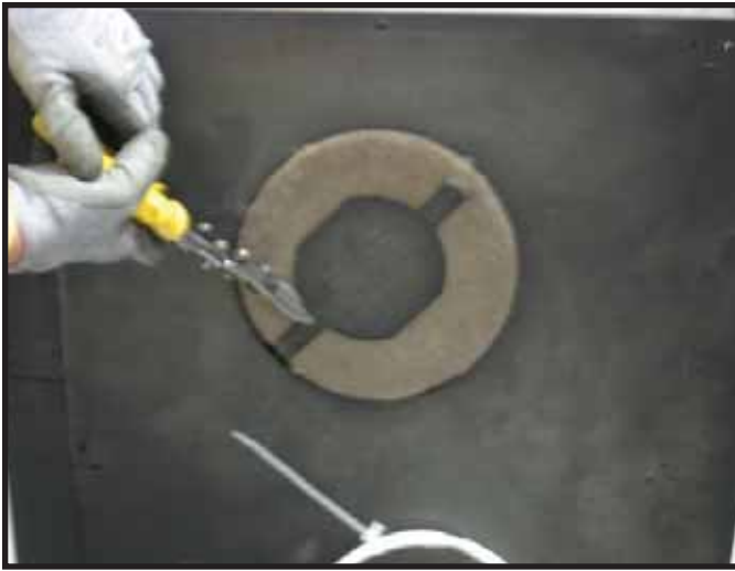
Figure 9.5 Cut the metal retaining band.
