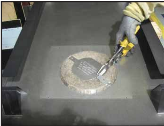
Figure 9.2 Cut the metal retaining band and fold the sides out.
