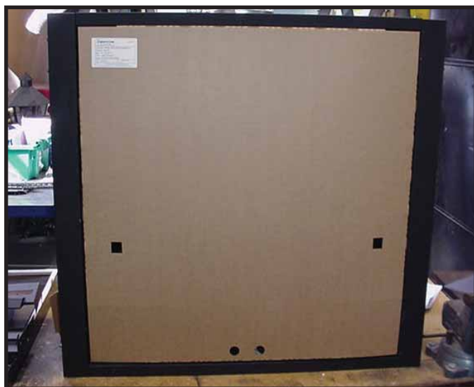
Figure 13.11 Splatter Guard with Lower Access Panel Closed
