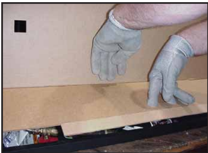
Figure 13.8 Opening Lower Access Panel
