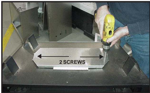
Figure 16. For top flue, remove the two screws holding the top heat shield in place. For rear flue, see next page.
