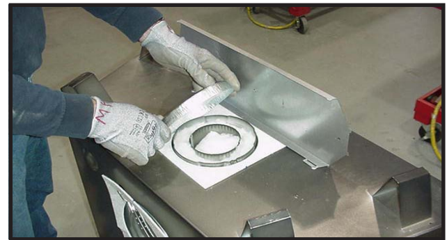
Figure 19. Remove the flue cap.
