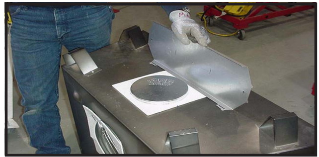
Figure 17. Rotate the top heat shield to the vertical position as shown above. The heat shield must remain in the vertical position.
