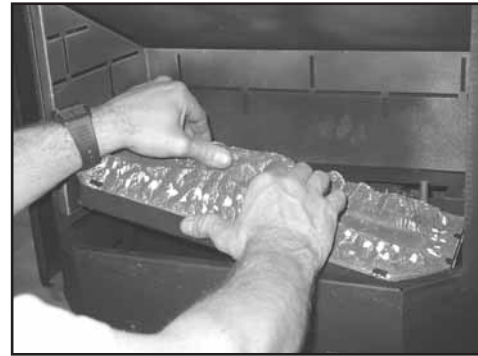
Figure 6.2 Lift the burner from the left side and slide left until free from the orifice receiver. Remove from the firebox and handle with care.
