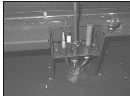
Figure 6.4 Remove the pilot hood, and set aside. Using a 5/32 in. allen wrench, remove the pilot injector and replace with an appropriate injector (35 LP, 62 NG).
