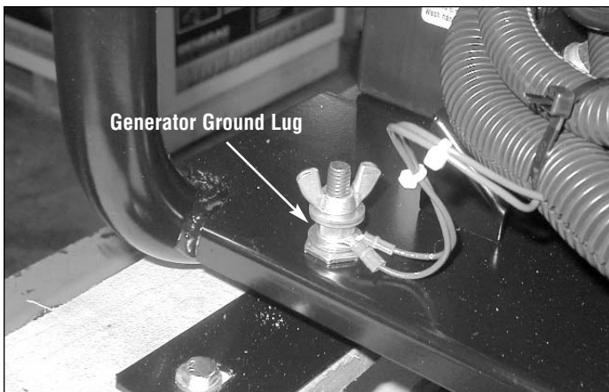
Figure 13 - Grounding the Generator
