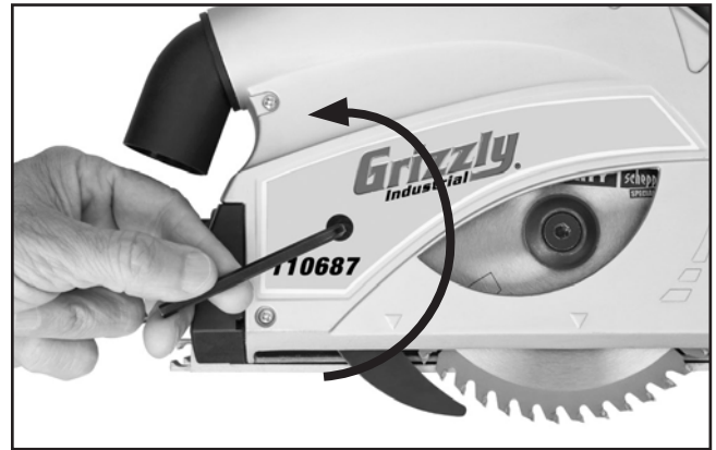
Figure 13. Loosening the riving knife lock.
