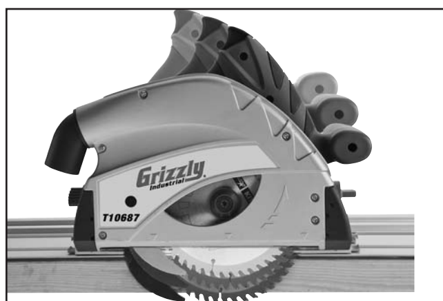
Figure 20. Plunge-action lowering for the cut.
