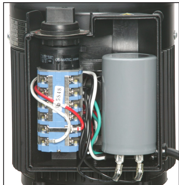
Figure 19. Motor switch and capacitor (front view).
