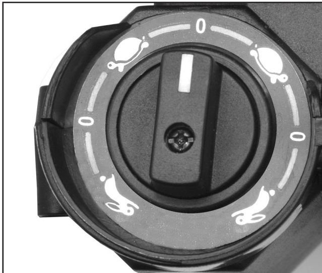
Figure 13. Feed direction and speed dial.
