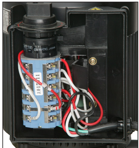
Figure 21. Motor switch (front view).
