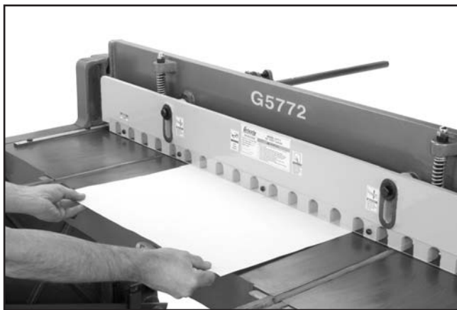
Figure 28. Example of a paper shear test.
