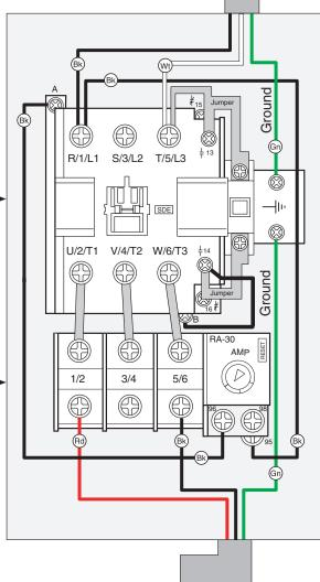
**IMPORTANT:** This magnetic switch toggles a motor ON and OFF, and helps provide thermal overload protection for the motor if operating temperature gradually increases due to heavy work loads. The thermal overload relay inside is not designed to cut power in the event of a sudden motor overload or stall.
