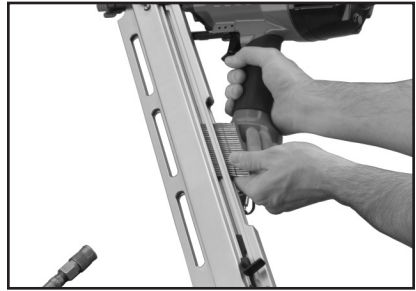
Figure 4. Loading nails into the magazine.
