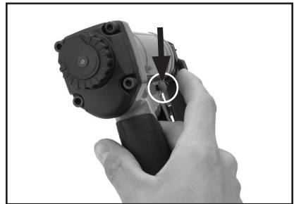
Figure 6. Trigger switch, single fire mode.
