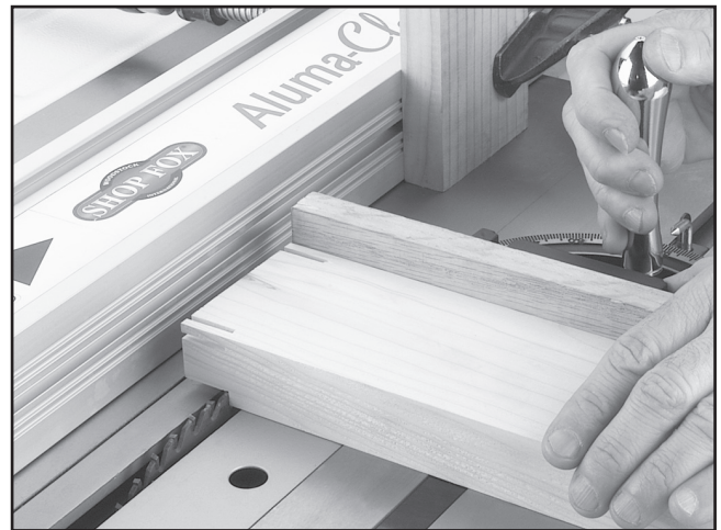
Figure 26. Cutting the shoulder.
