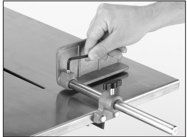
Figure 17. Securing fence to rail.
