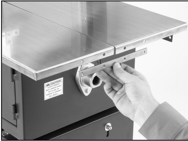
Figure 13. Attaching table brace.
