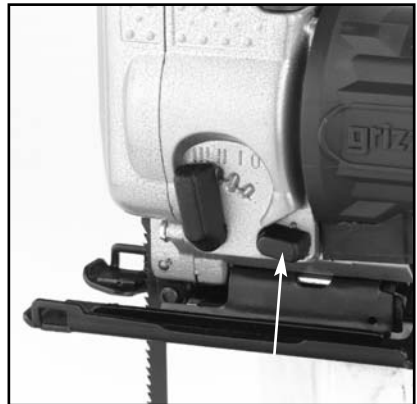
Fig 7. Chip blower switch.
