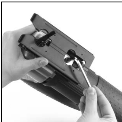
Fig 9. Setting footplate for angle cuts.
