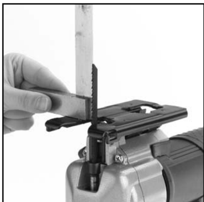
Fig 8. Checking blade squareness.
