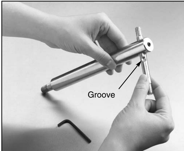
Figure 9. Slide bar into guide shaft.
