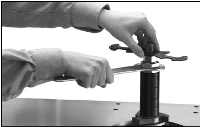
Figure 33. Tightening spindle nuts.
