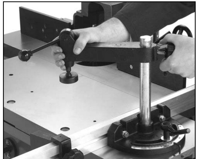
Figure 25. Installing the clamping unit.
