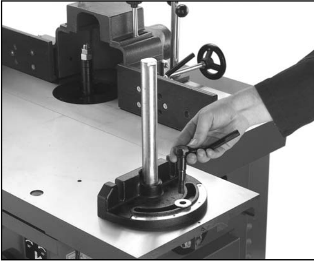
Figure 22. Installing the adjustable handle.
