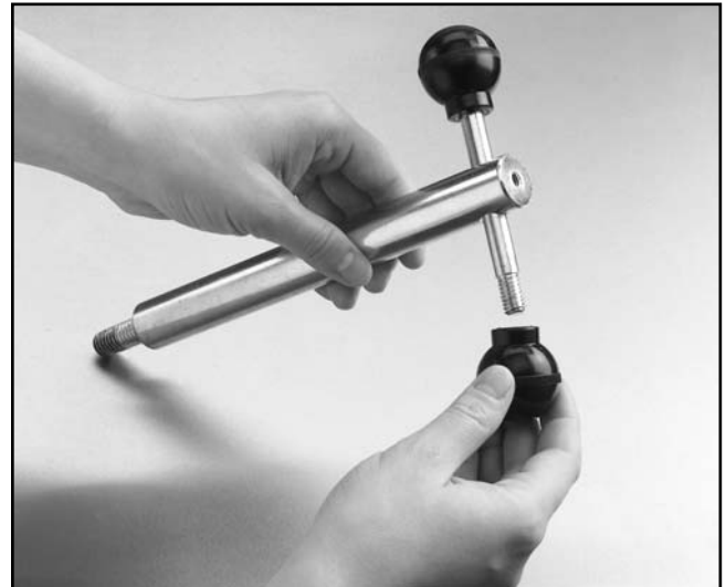
Figure 11. Thread round knobs onto bar.
