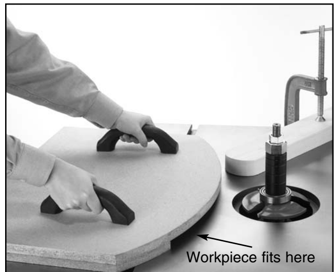
Figure 44. Pattern jig for making curved pieces (guard removed for clarity).
