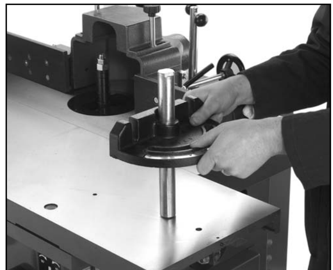
Figure 21. Installing the miter gauge. G8622 Tilting Spindle Sliding Table Shaper
