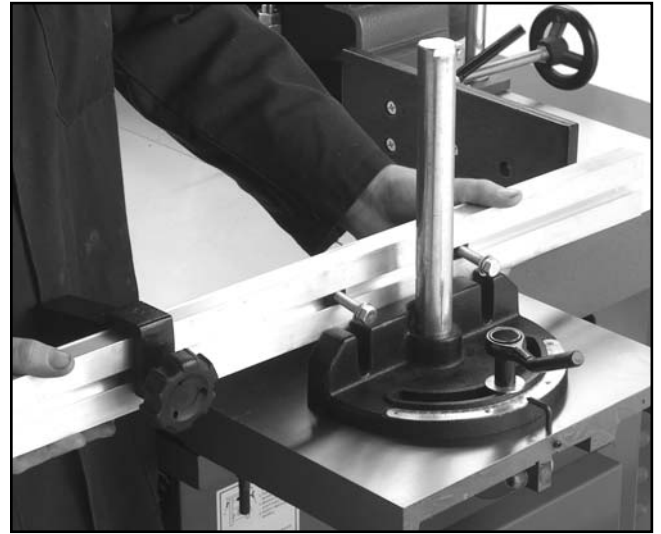
Figure 24. Installing the miter fence.
