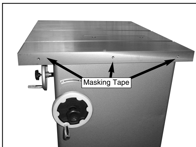
Figure 7. Using tape to shim for wing alignment.
