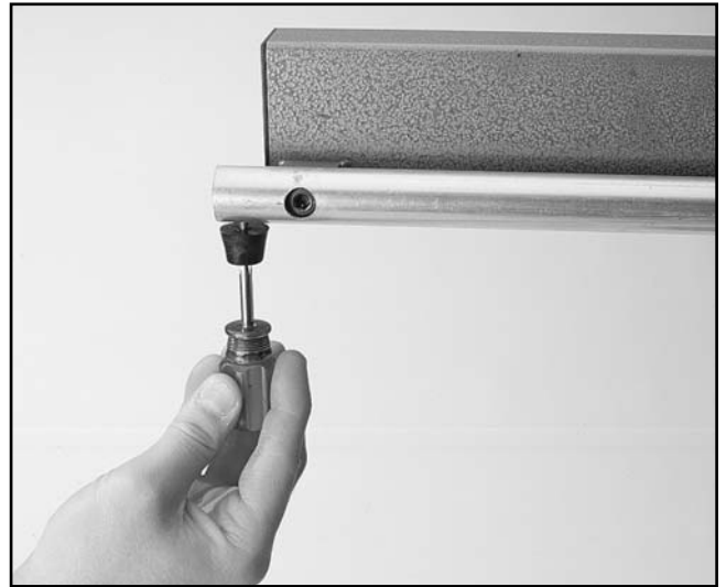
Figure 10. Rear stop installation.
