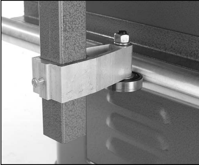
Figure 8. Adjust lower guide bearing.
