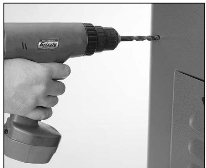
Figure 3. Drilling the mounting holes.
