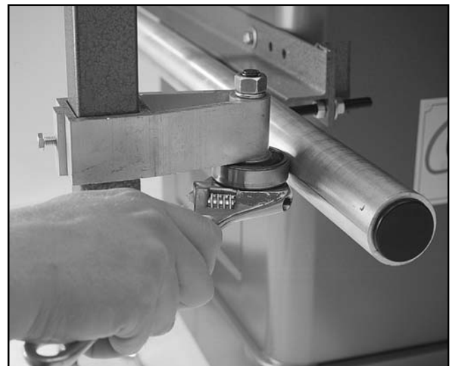
Figure 15. Adjusting the lower guide.
