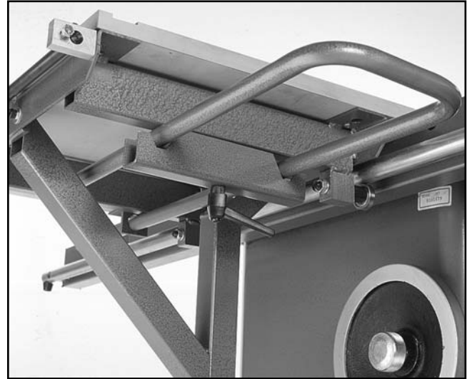
Figure 18. Installing auxiliary handle.
