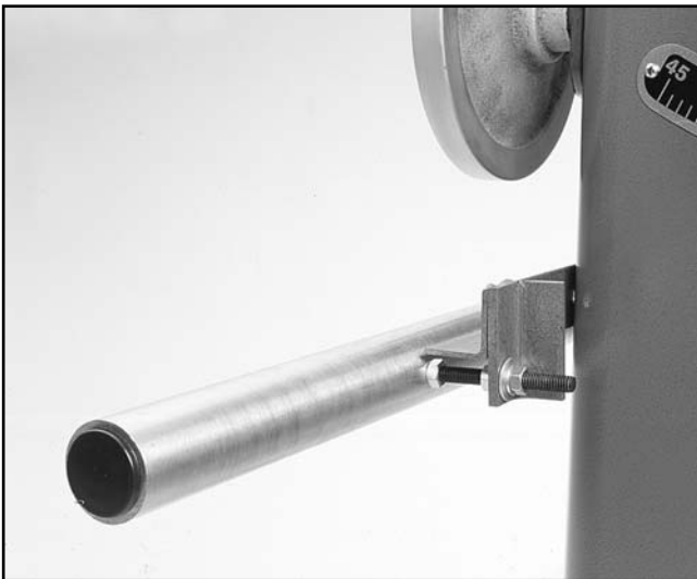
Figure 5. Mounting the lower rail.
