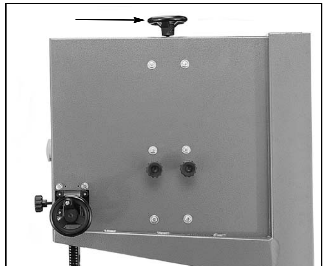
Figure 27. Tension control knob.
