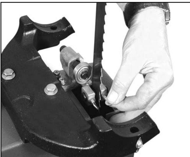
Figure 4. Installing blade guide assemblies.
