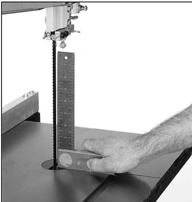
Figure 20. Checking blade to table.
