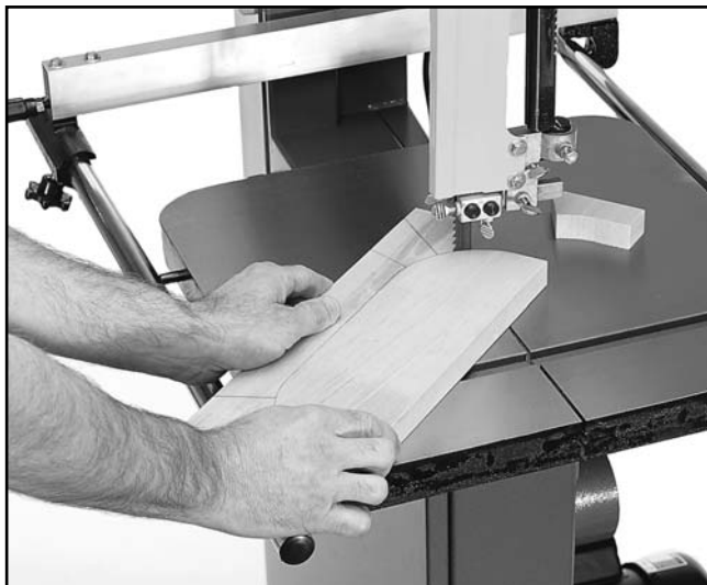
Figure 29. Typical curve cutting operation.
