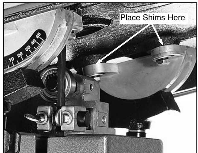
Figure 21. Front to back shimming.
