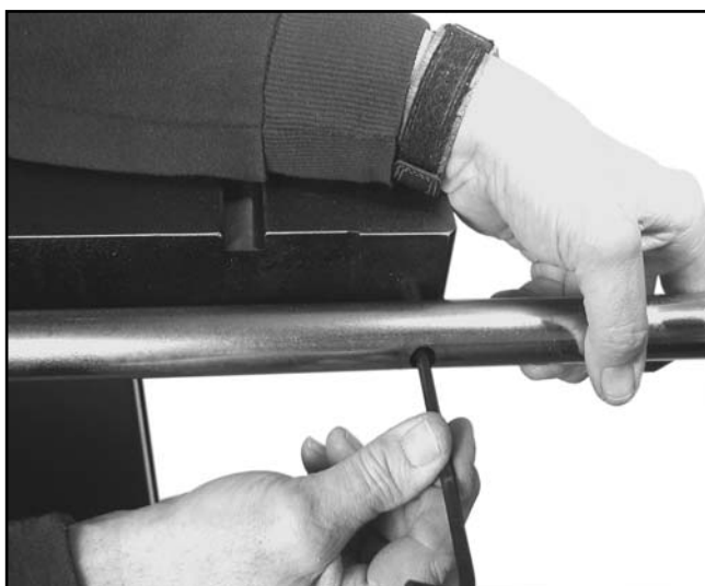
Figure 7. Securing the rail to the table.
