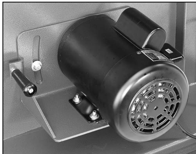
Figure 23. Motor mounting plate.
