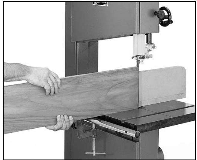
Figure 30. Resawing with an auxiliary fence.
