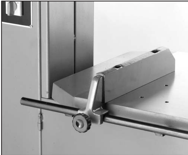
Figure 5. Fence mounted on rail.
