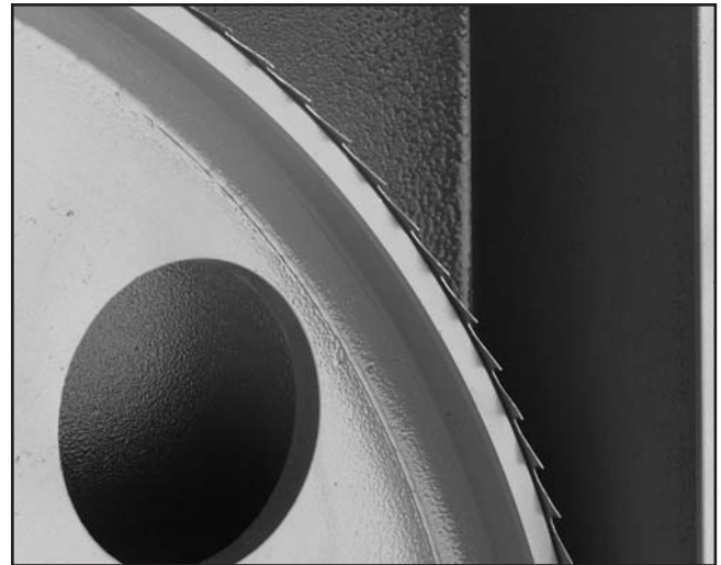
Figure 10. Bottom of teeth gullets protruding \frac{1}{16} " from the edge of the upper wheel.
