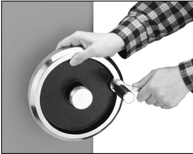
Figure 15. Tightening handle onto handwheel.
