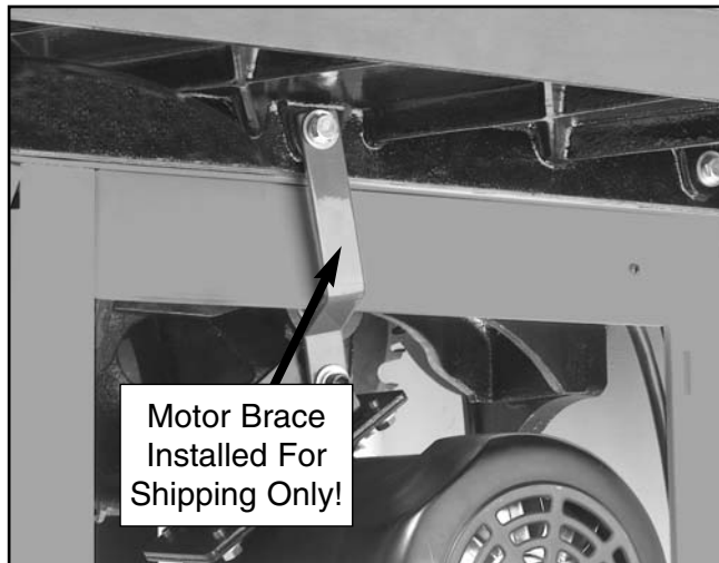
Figure 12b. Motor brace.
