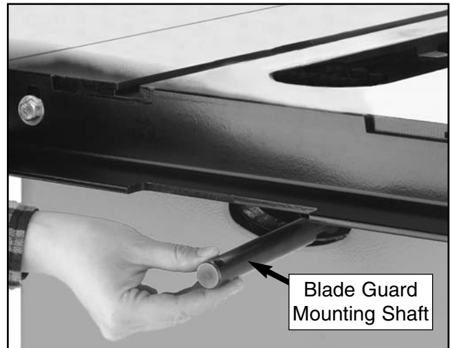
Figure 13. Attaching the \frac{5}{8} "-18 blade guard mounting shaft.
