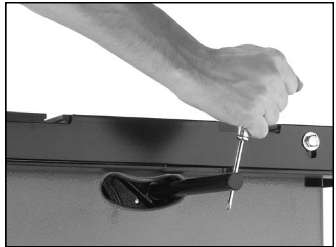
Figure 12. Attaching guard support shaft.
