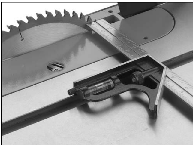
Figure 24. Adjusting blade to miter slot.
