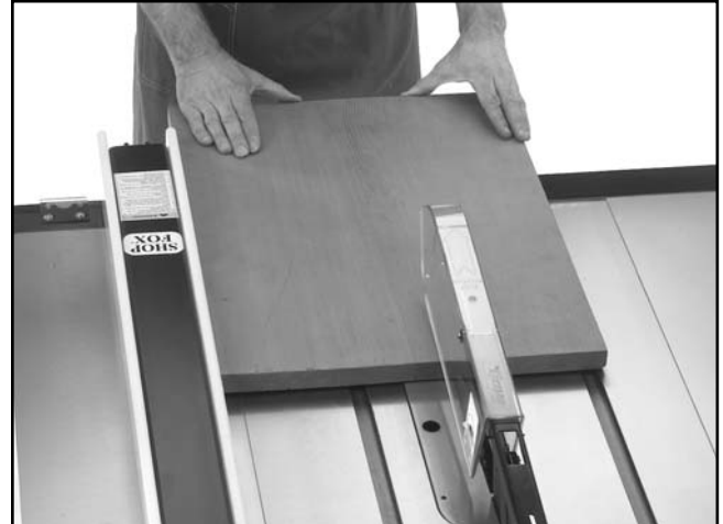
Figure 37. Do not stand directly behind wood!
