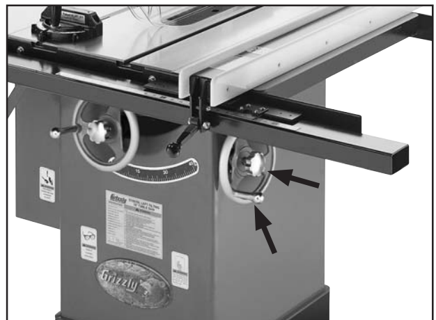
Figure 24. Handle and lock knob installed on handwheel.
