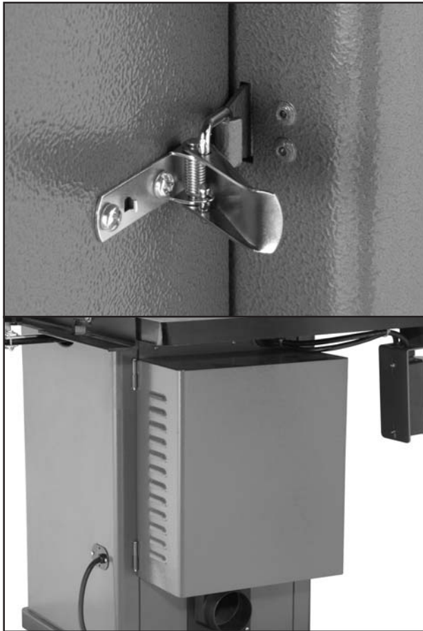
Figure 22. Motor cover installed on stand.
