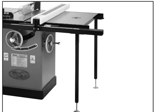
Figure 18. Router table and legs installed.
