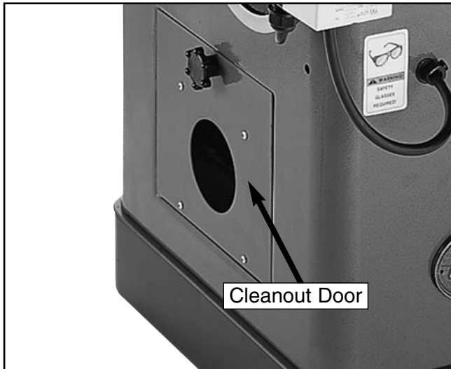
Figure 11a. Installed cleanout door.
