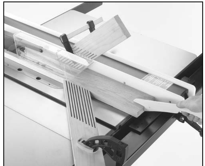
Figure 31. Typical ripping operation.
