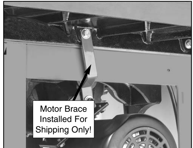
Figure 11b. Motor brace.
