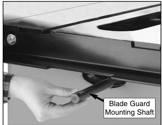
Figure 12. Attaching the \frac{5}{8} "-18 blade guard mounting shaft.
