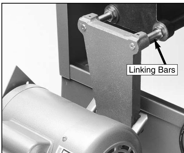
Figure 19. Attaching motor to linking bars.
