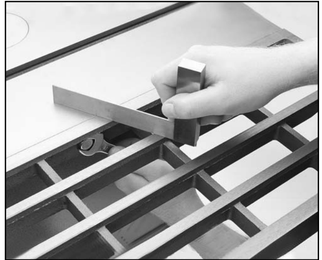
Figure 23. Checking table to wing alignment.
