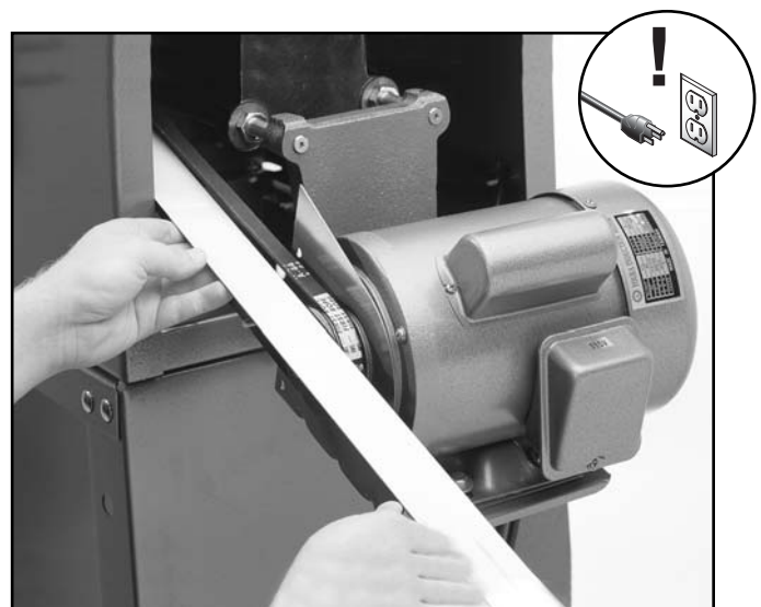
Figure 21. Checking V-belt alignment.
