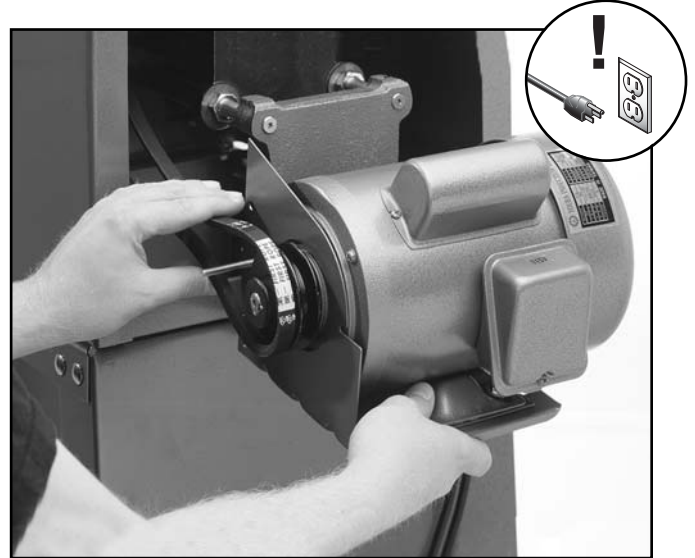
Figure 20. Attaching the V-belt to the motor.
