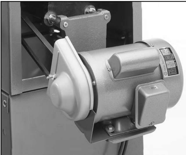
Figure 20. Attaching the pulley guard.
