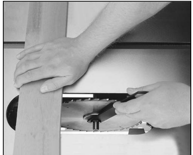
Figure 24. Changing saw blade.
