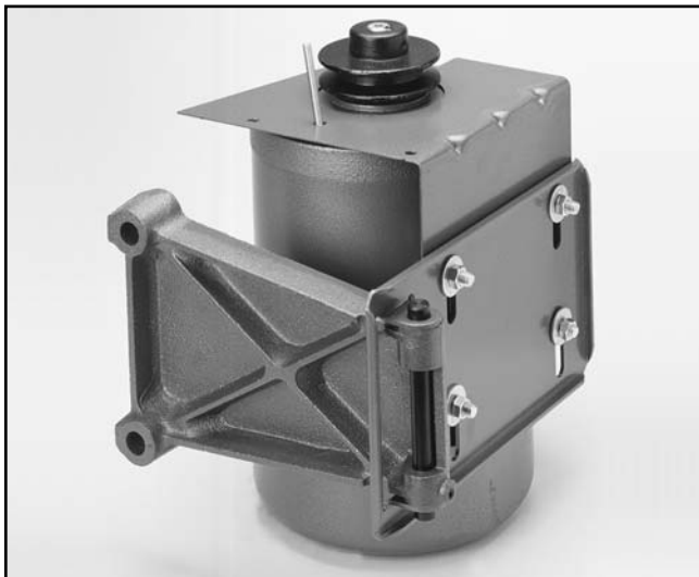
Figure 16. Installing the motor mount bracket.
