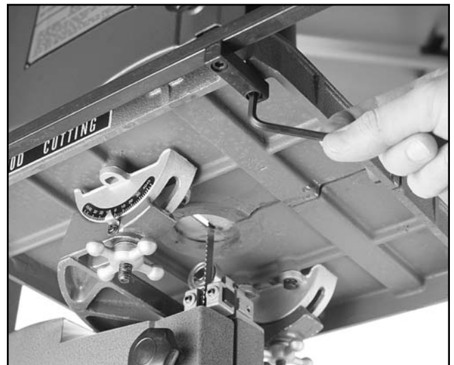
Figure 21. Fence rail bracket attachment.
