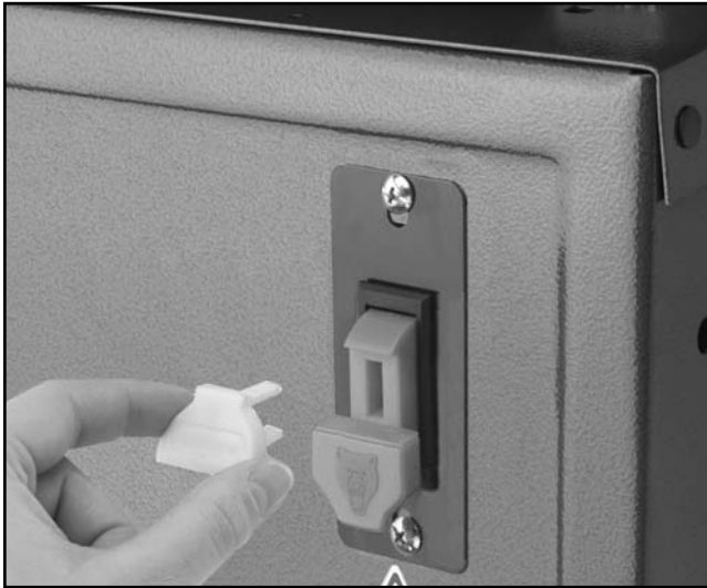
Figure 12. Removing lock-out key from switch.
