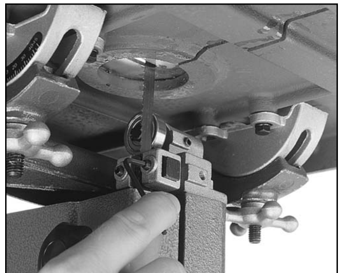
Figure 26. Lower blade guide assembly.
