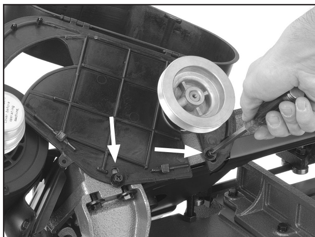
Figure 13. Installing pulley cover.
