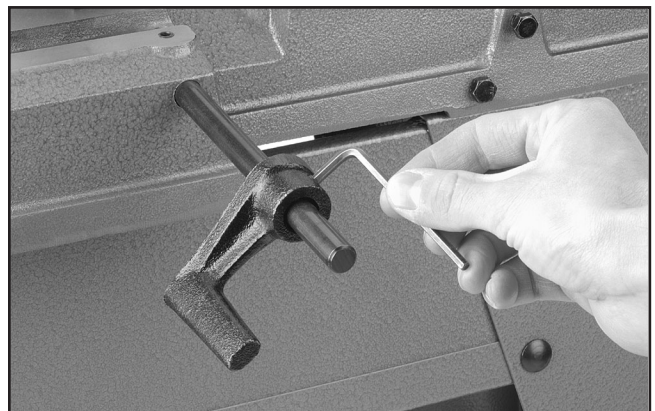
Figure 19. Installing work stop.
