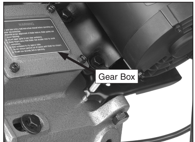
Figure 45. Gear box lubrication.
