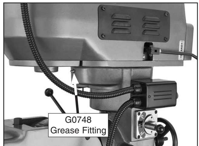
Figure 55. Model G0748 headstock gearing grease fitting.
