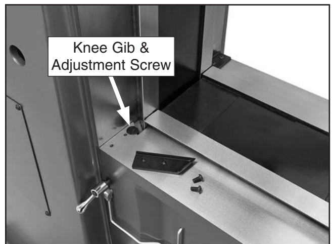
Figure 64. Knee gib and adjustment screw.
