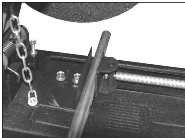
Figure 12. Example photo of workpiece held firmly between the vise jaws.
