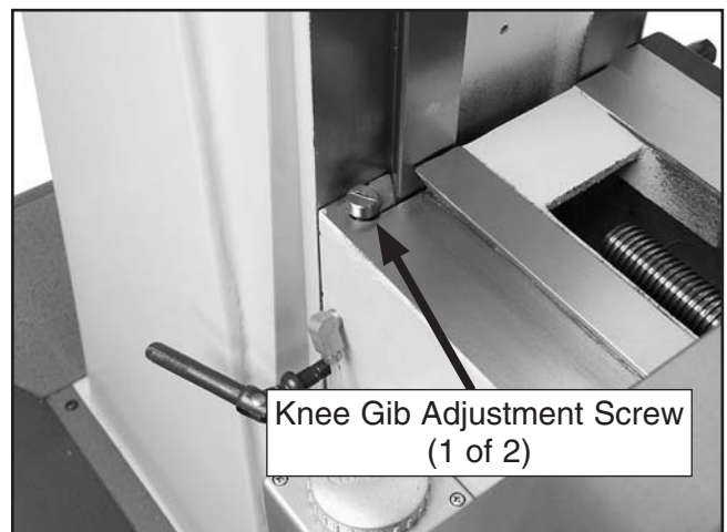
Figure 54. Knee gib adjustment screw (1 of 2).
