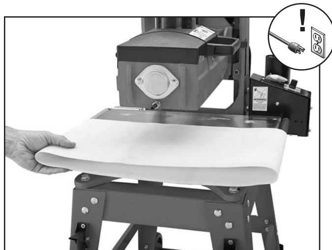
Figure 40. Removing the conveyor belt.
