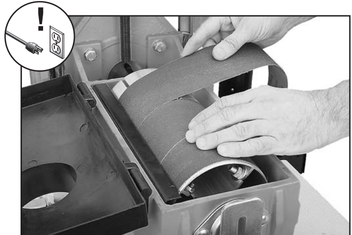
Figure 20. Wrapping sandpaper strip on the drum.
