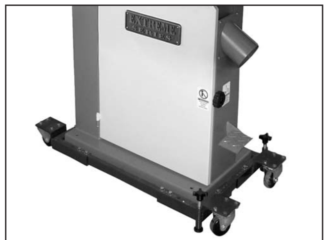
Figure 10. Bandsaw mounted on a G7315Z SHOP FOX® Mobile Base.
