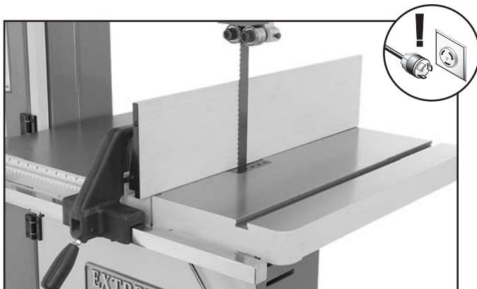
Figure 30. Fence against the blade.
