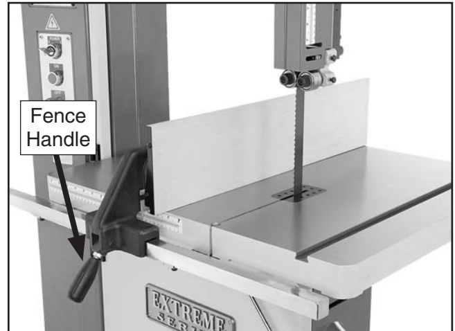
Figure 20. Fence assembly mounted on the fence rail.
