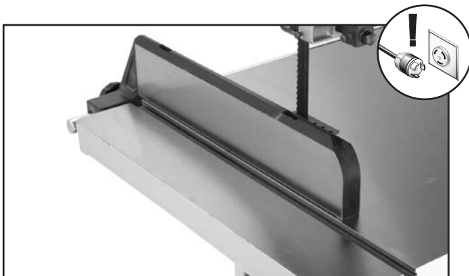
Figure 28. Fence even with the miter slot.
