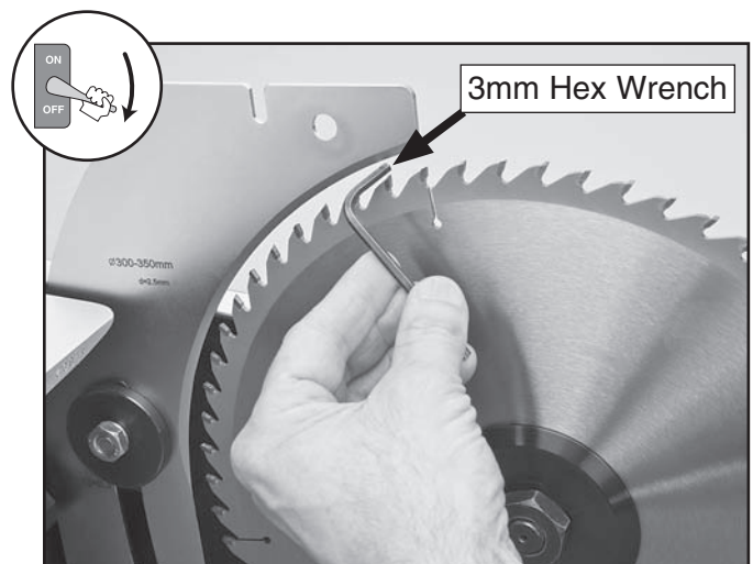
Figure 70. Setting the correct riving knife spacing.
