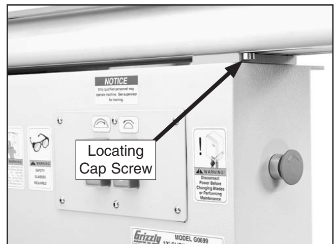
Figure 21. Sliding table locating cap screw against the right side of the frame.
