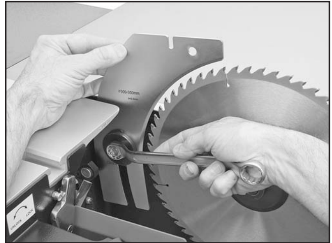
Figure 16. Installing the riving knife.
