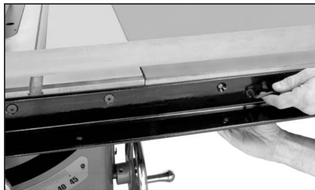
Figure 31. Aligning main extension table.
