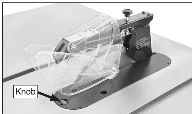
Figure 64. Blade guard and insert installed.
