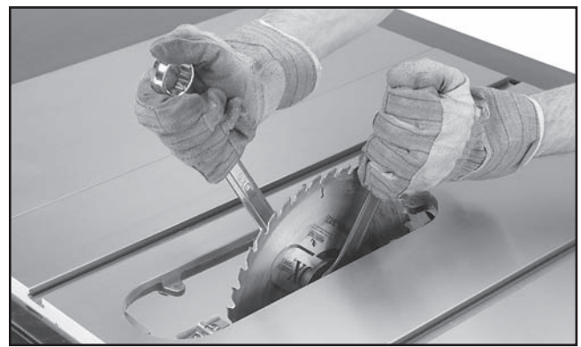
Figure 60. Loosening arbor nut.
