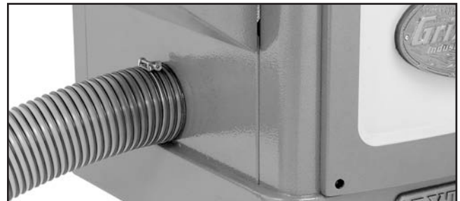
Figure 44. Dust hose attached to dust port.
