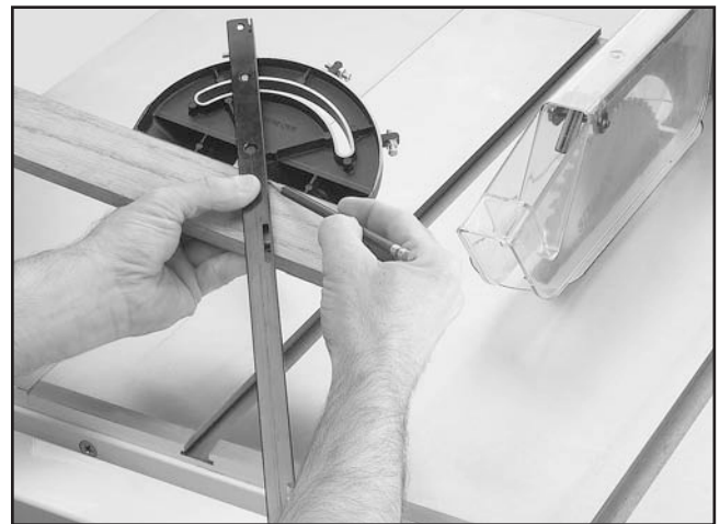
Figure 75. Example of marking miter line.
