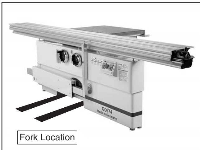
Figure 11. Lifting the saw base unit.
