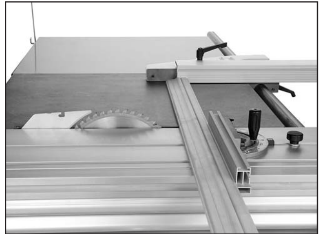
Figure 70. Crosscutting workpieces using the rip fence as a cut-off gauge (blade guard removed for clarity).
