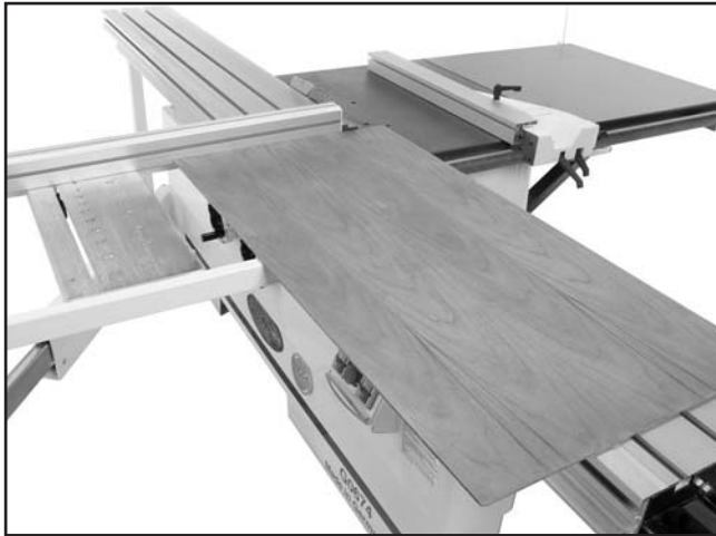
Figure 61. Rip cutting with the sliding table.
