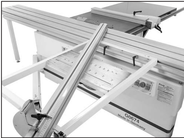
Figure 73. Fence set-up for 90° to 135° cuts.
