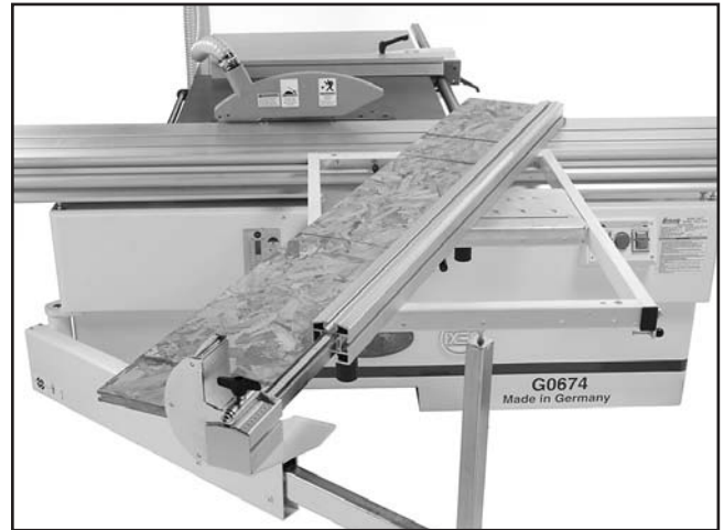
Figure 74. Example of miter cutting operation.
