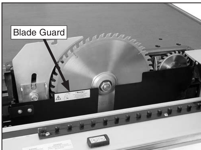
Figure 50. Internal blade guard exposed.
