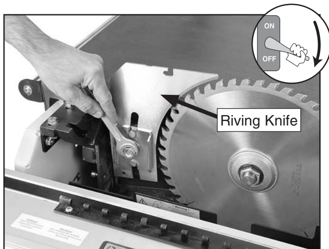
Figure 55. Re-adjusting the riving knife.
