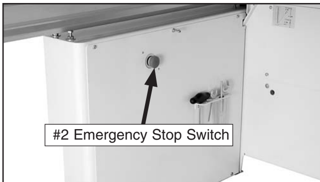
Figure 38. Emergency stop switch #2.
