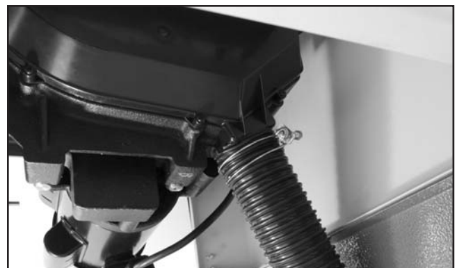
Figure 27. Dust hose attached to dust port.
