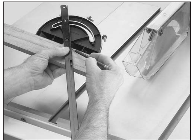
Figure 44. Example of marking miter line.
