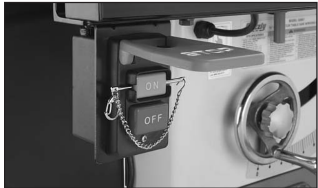
Figure 28. Switch disabling pin inserted into ON button.
