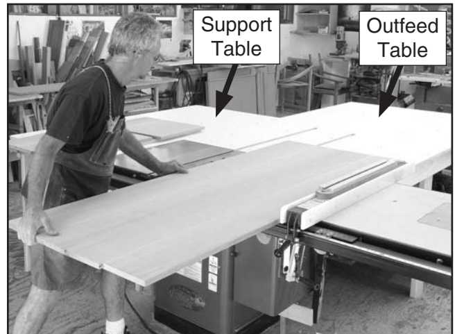
Figure 72. Example of outfeed & support tables.
