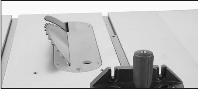
Figure 45. Blade tilted to 45° for bevel cutting on a typical table saw.
