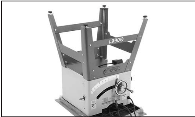
Figure 12. Stand assembly positioned on saw.
