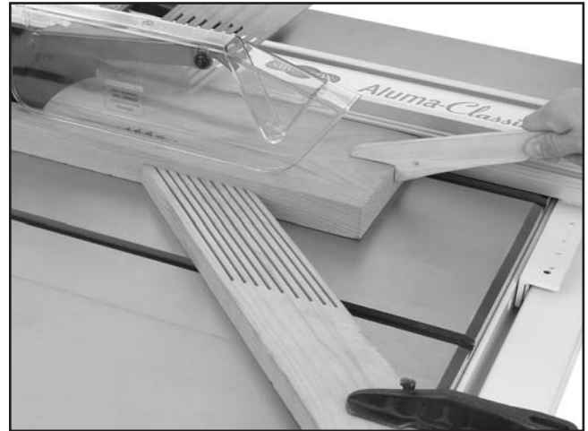
Figure 42. Typical ripping operation.
