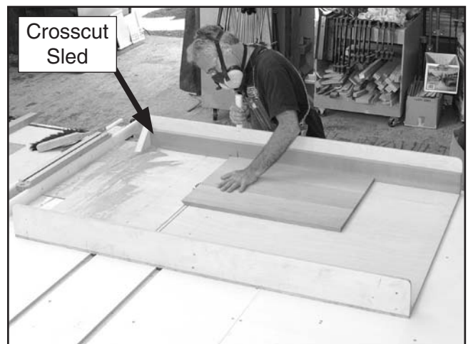
Figure 73. Example of crosscut sled.
