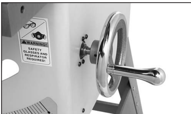
Figure 13. Handwheel installed on side of saw.
