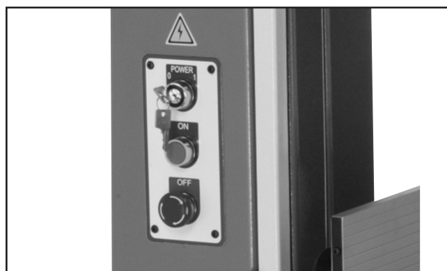
Figure 4. G0636XB switch disabling key and ON/OFF switch.
