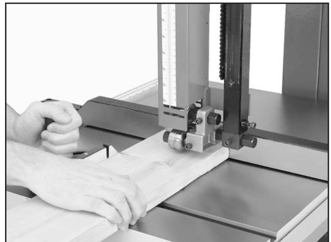
Figure 33. Typical crosscutting operation.
