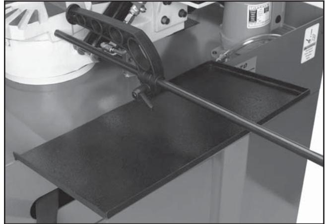
Figure 20. Splash tray installation.
