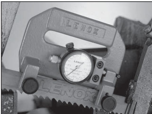
Figure 24. H5408 Blade Tensioning Gauge.
