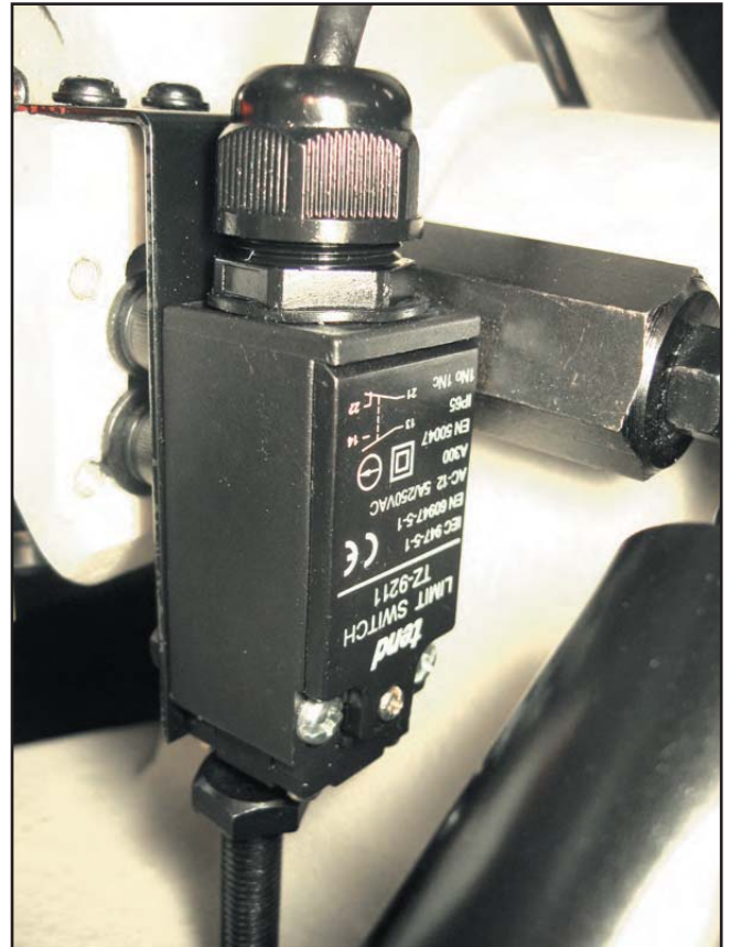
Figure 72. G0614 blade stop limit switch.
