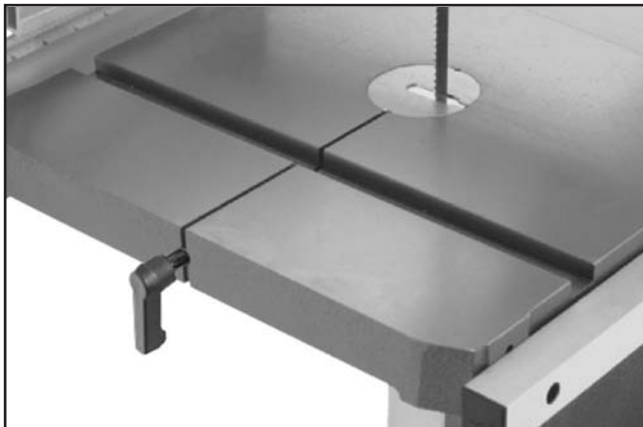
Figure 20. Table pin and insert installed.
