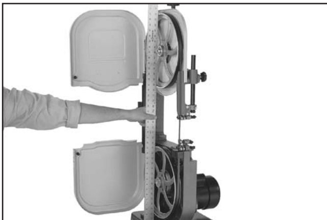
Figure 68. Checking if the wheels are coplanar.
