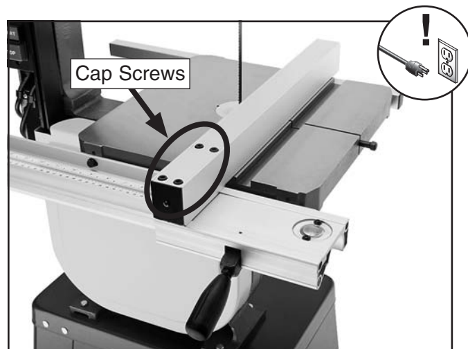
Figure 41. Location of the fence adjustment cap screws.
